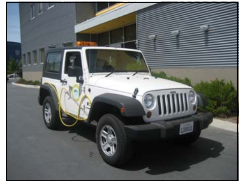
Right-hand drive Jeep used to treat catch basins and storm drains
